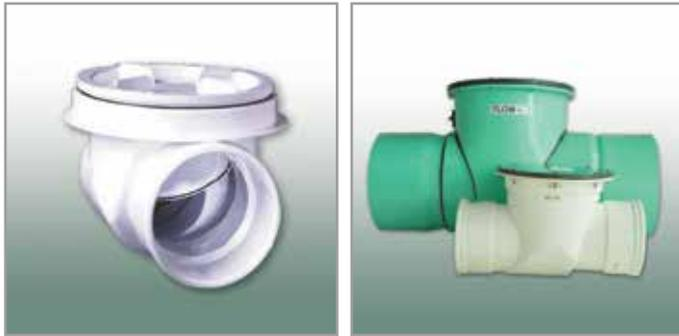
Backwater Valves ensure one-way flow in storm and sanitary sewer lines where backflow could be a problem. In a municipal Right of Way, we offer two types of Backwater Valves, in-line and terminal. Each Backwater Valve is equipped with a flapper that allows unrestricted flow. The flapper remains closed protecting against backflow and opens only when there is flow from the system.
