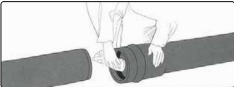
Figure 2 Cleaning gasket and bell.
