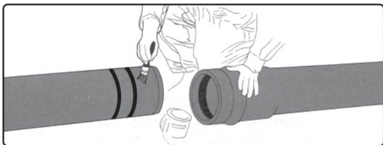
Figure 3 Apply lubricant.
